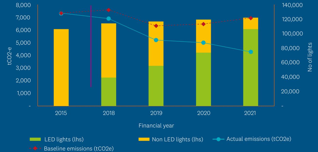
Figure 3: An indicative contribution of GHG emissions reduction due to LED retrofit.
