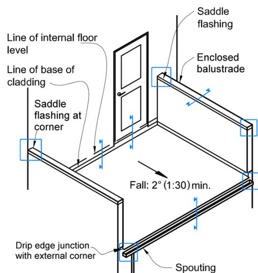
Membrane decks, roofs and gutters have a high occurrence of weathertightness failure. Often this can be due to surfaces having been constructed with minimal falls, tiles having been fixed directly to the membrane, and perimeter junctions and walls lacking adequate flashing. Membranes have also failed due to movement in substrates, age and/or poor maintenance.
