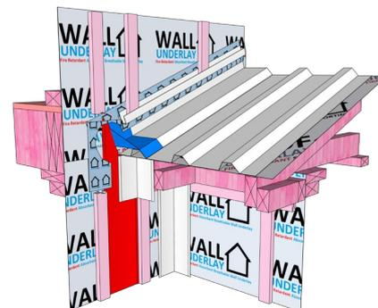
**Step 3:** Overlap wall underlay from above, flashing tape and cavity battens
