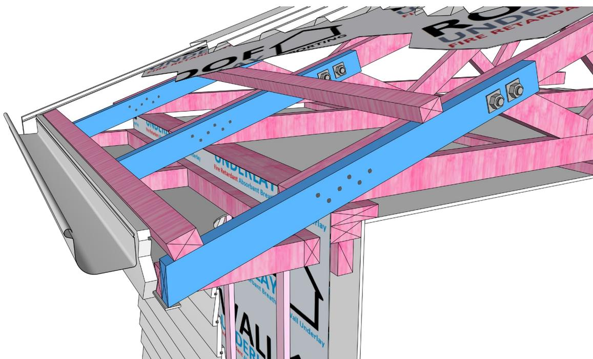
Flitching new framing to a truss top chord or rafter to create an eaves overhang
