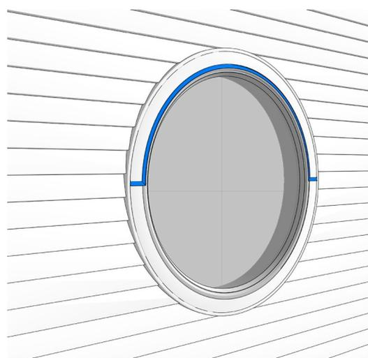
Round window flashing requires alternative solution design detailing
