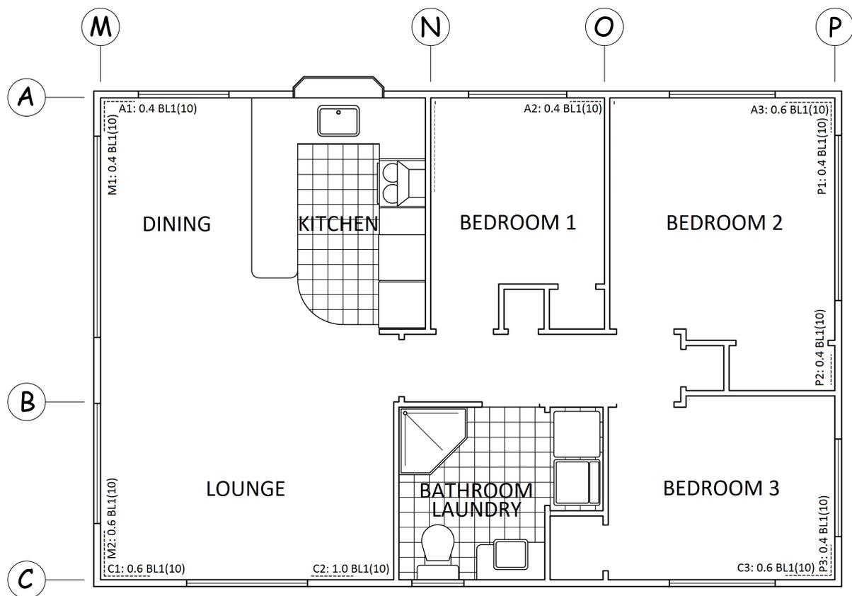
Wall bracing layout plan specifying brace element type and length
