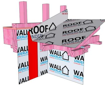
**Step 1:** Back flashing, wall and roof underlay
