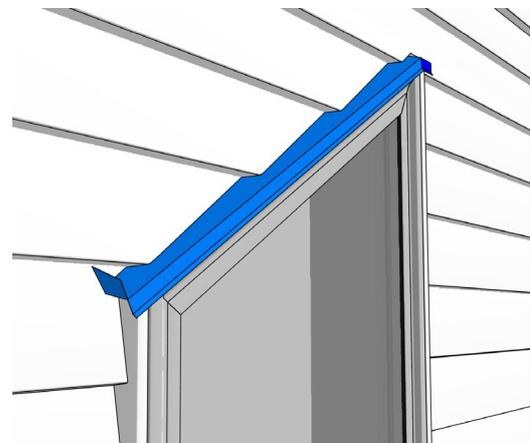
Raked window head flashing – fully welded
