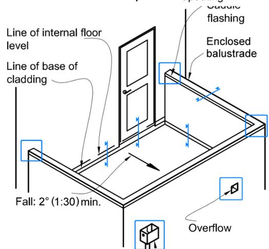
Gutter or low point of roof to discharge through scupper to rainwater head or roofing outlet
