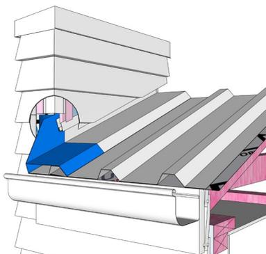
Gutter/fascia junction at parapet corner
