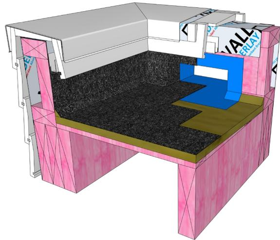
Membrane applied into preformed scupper
