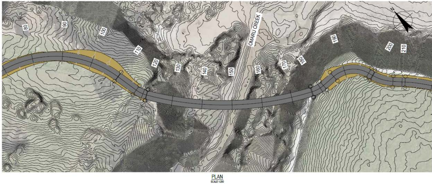
Figure 12: Proposed plan drawing of Omaru Creek Bridge (GHD, 2016)
