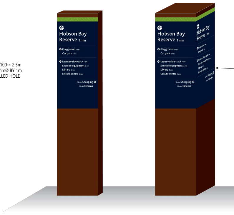
4 SINGLE AND DOUBLE WAYFINDING BOLLARD NTS
