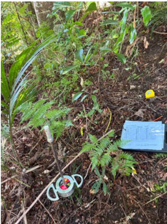
Picture 15: Hand Auger, Scala 4 Test Area
