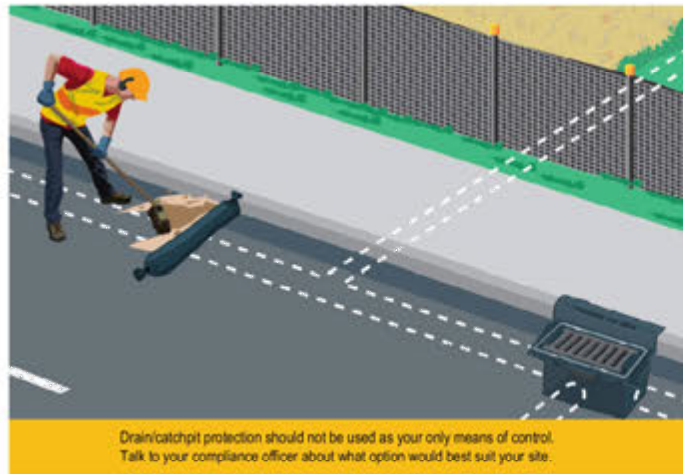
03 Drain/Catchpit Protection Sediment and erosion control guideline
