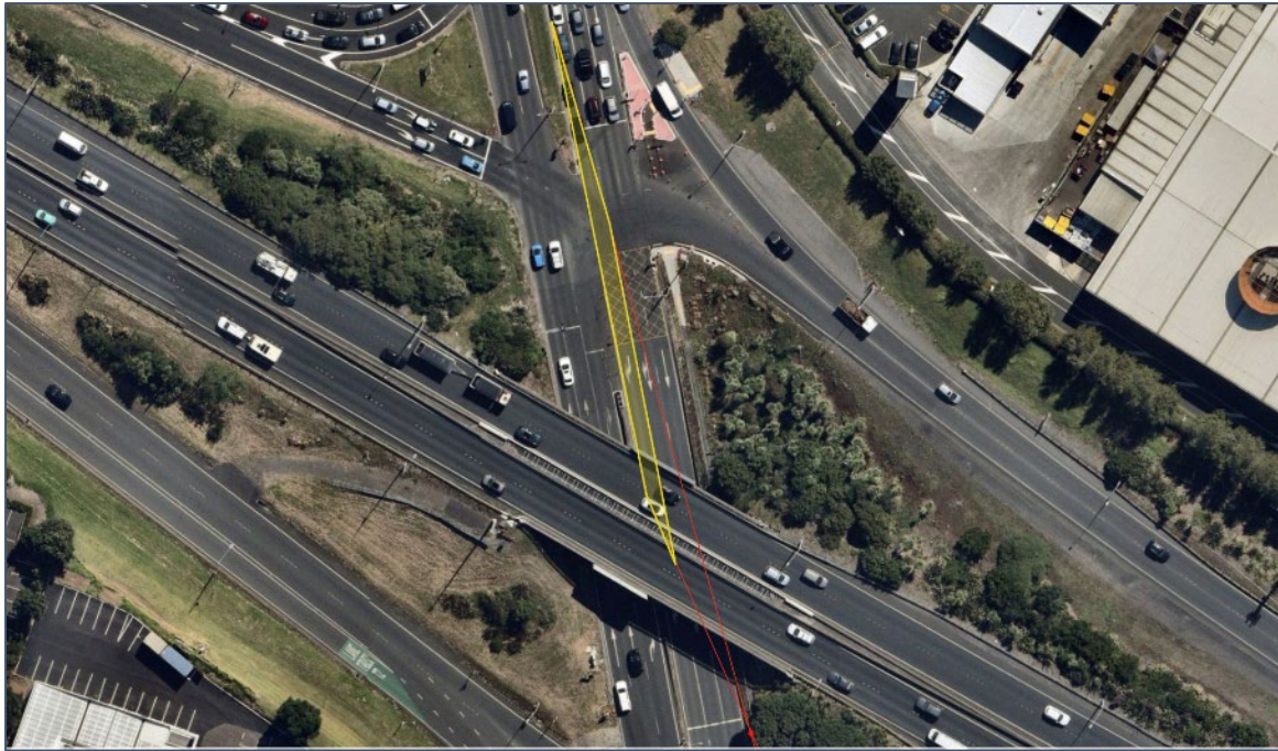
Figure 15: Projection from billboard through the primary signal into Lane 3
