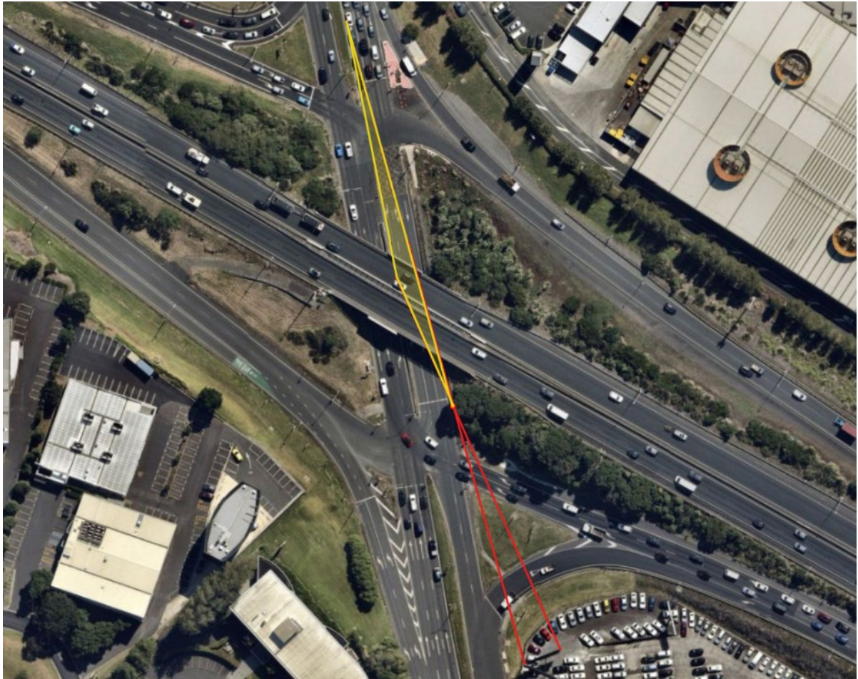
Figure 6: Projection from billboard through the primary signal to the southbound approach
