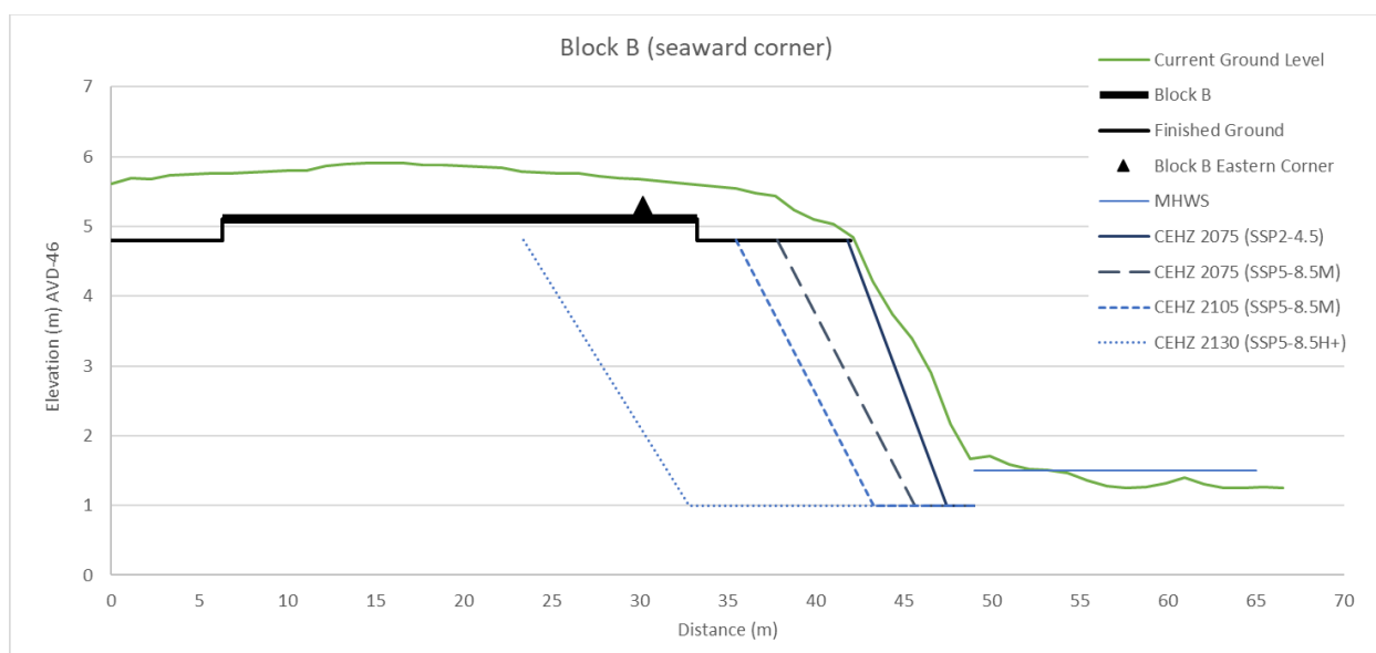
Figure 11: Coastal erosion hazard in relation to the ground floor of Block B.
