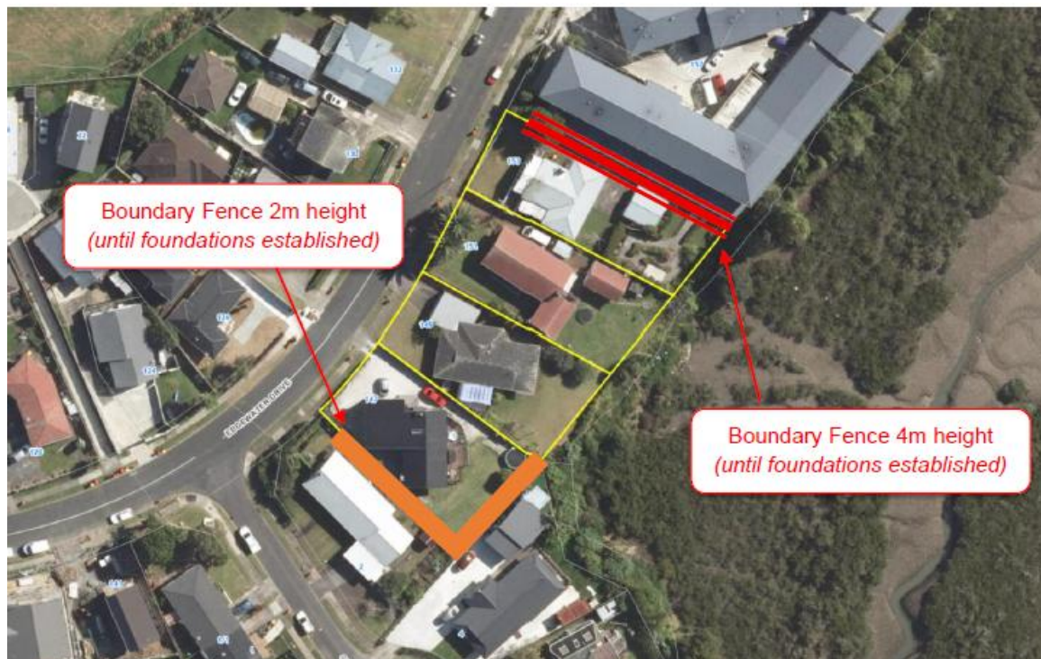
Figure 16: Proposed acoustic fencing which is to remain in place until foundations are established. Source: Earcon Construction Noise and Vibration Assessment
