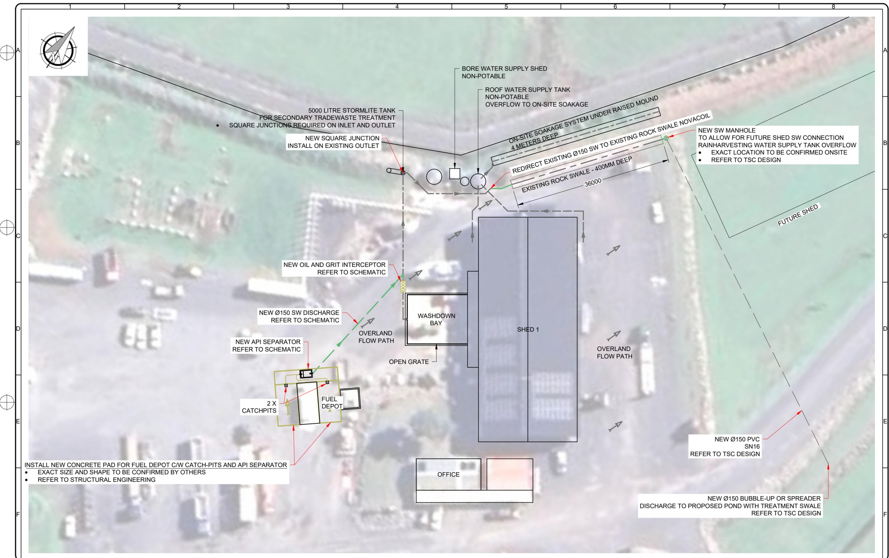
INSTALL NEW CONCRETE PAD FOR FUEL DEPOT C/W CATCH-PITS AND API SEPARATOR
