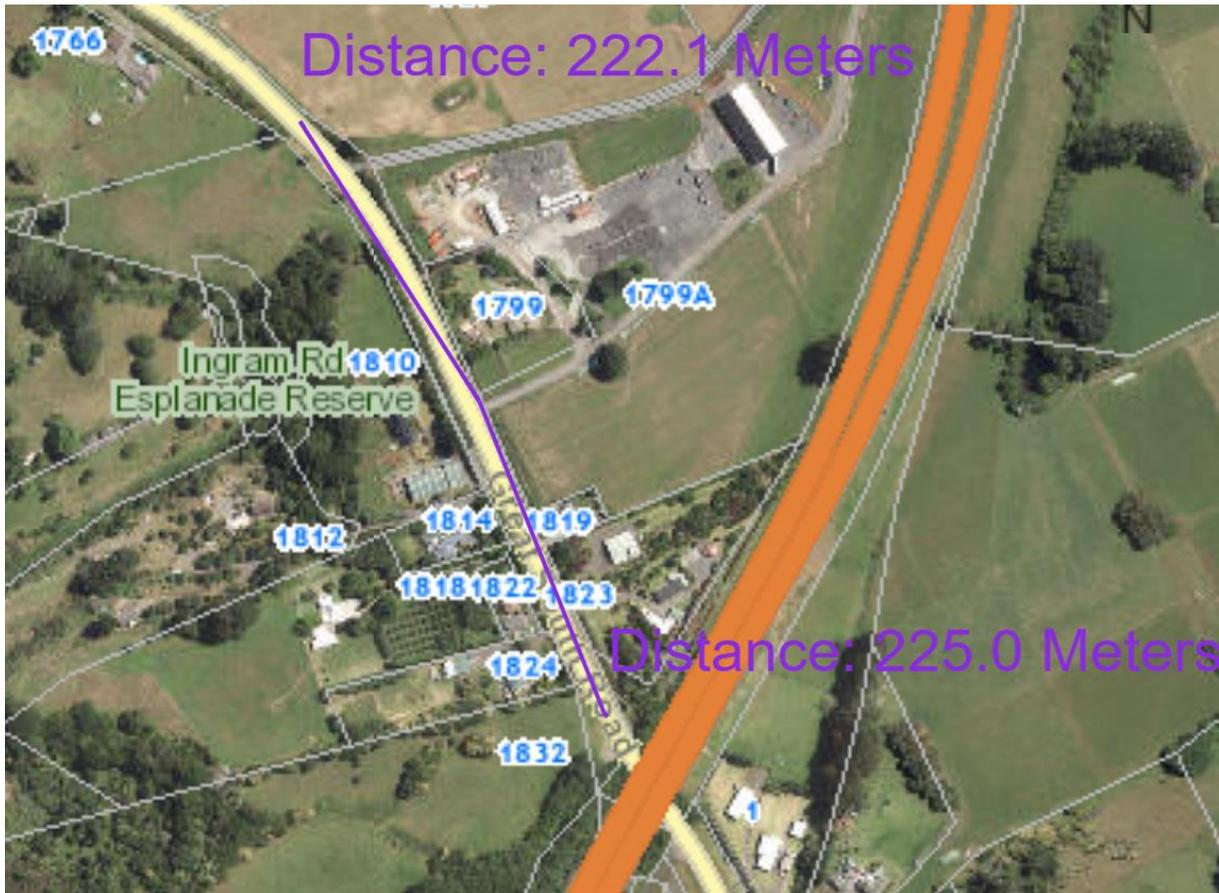
The diagram demonstrates that the available visibility exceeds the SISD requirement.
