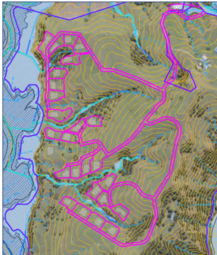
Figure 1: Proposed Lot Layout Overlaying the Flood Zones Taken from Auckland Council's 'GeoMaps' Application.
