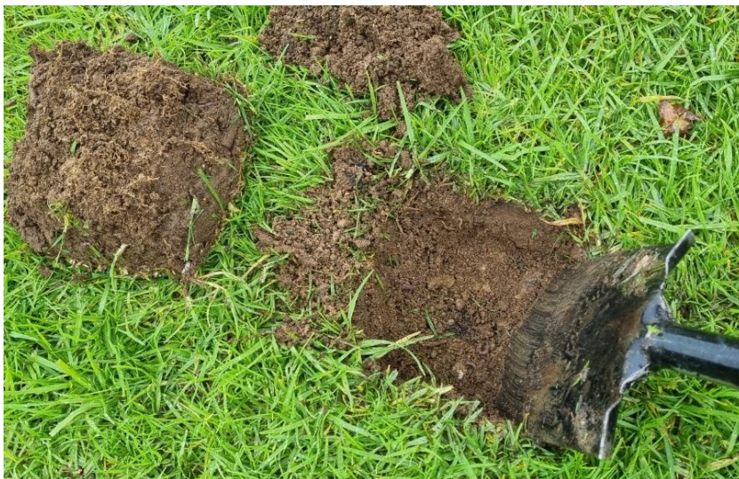
Figure 34. Subsurface testing within the grassed reserve at the southern end of Tui Street showing natural beach gravels below a thin layer of mid-brown topsoil.
