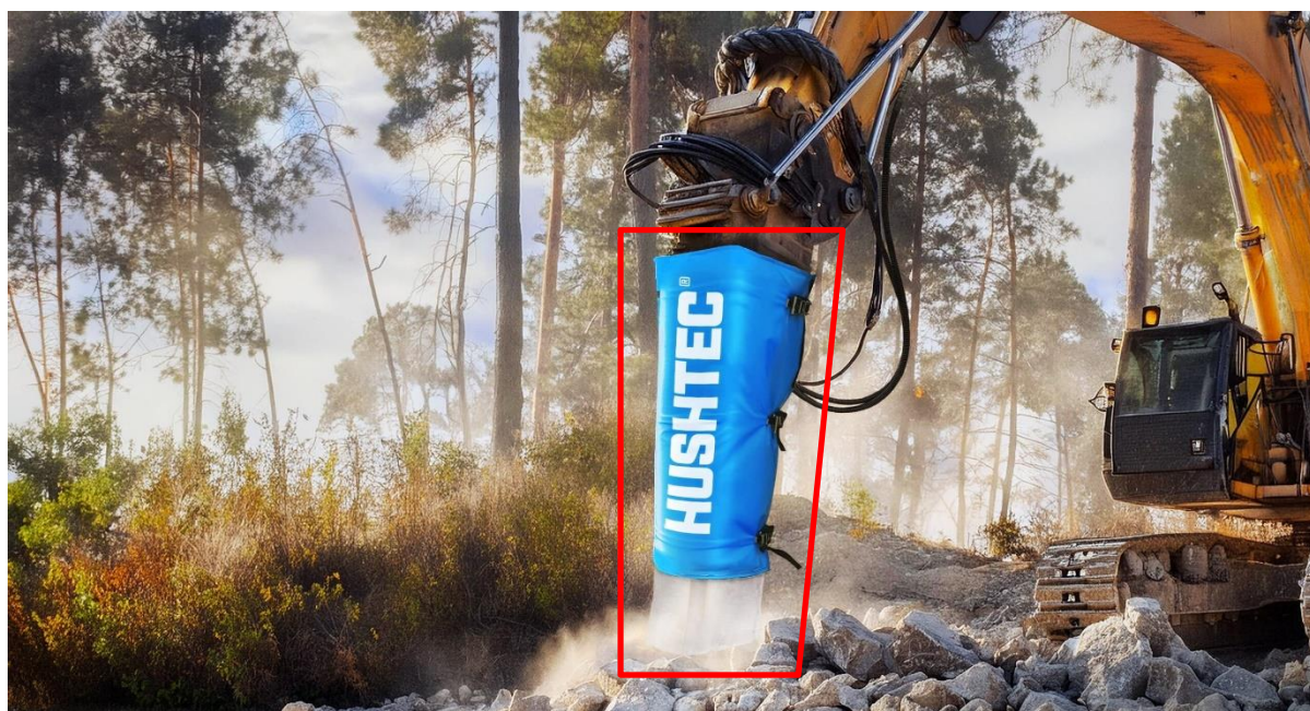
Figure 10 Example Setup of Acoustic Shroud Around Breaker Attachment
