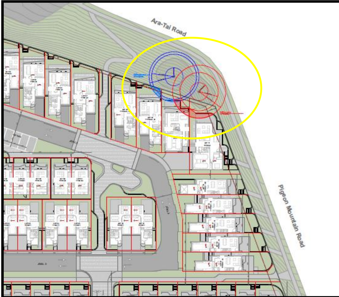
Figure 1 – Site plan showing location of trees in relation to overall site layout.
