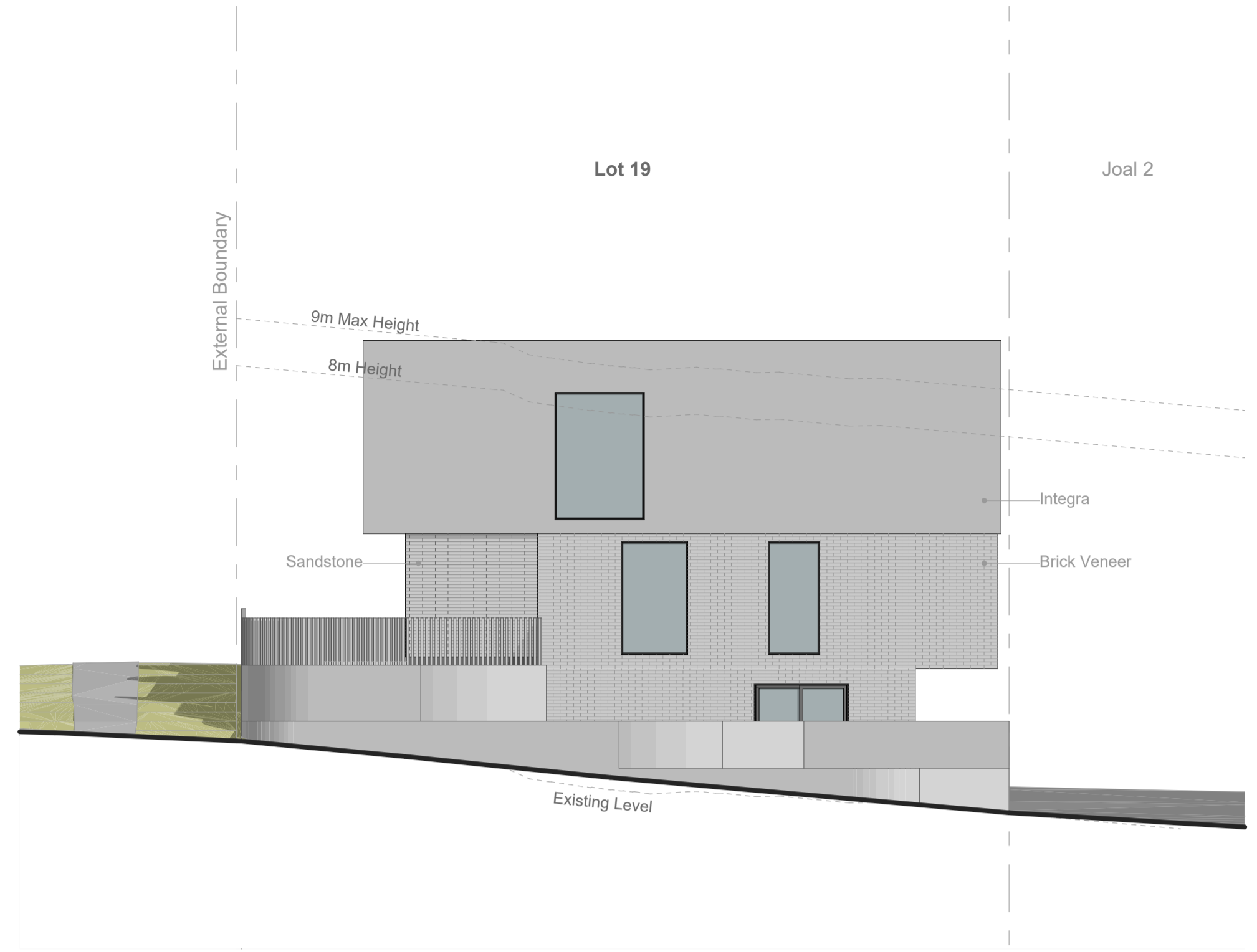
4 Block A - Elevation East 1:100
