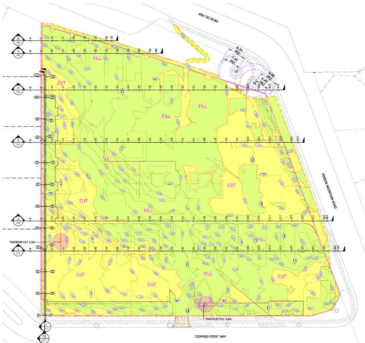
Figure 4: Cut to Fill Drawing (Source: Eighty6 Engineering)
