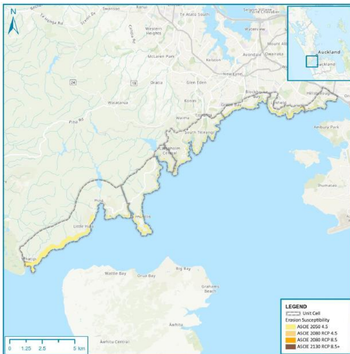
Figure 2-3: Coastal Instability and erosion susceptibility for 2050, 2080 and 2130 considering RCP4.5 and RCP8.5 emission scenarios Source: Manukau North Shoreline Adaptation Plan: Risk Assessment Technical Report, 2024, Tonkin & Taylor
