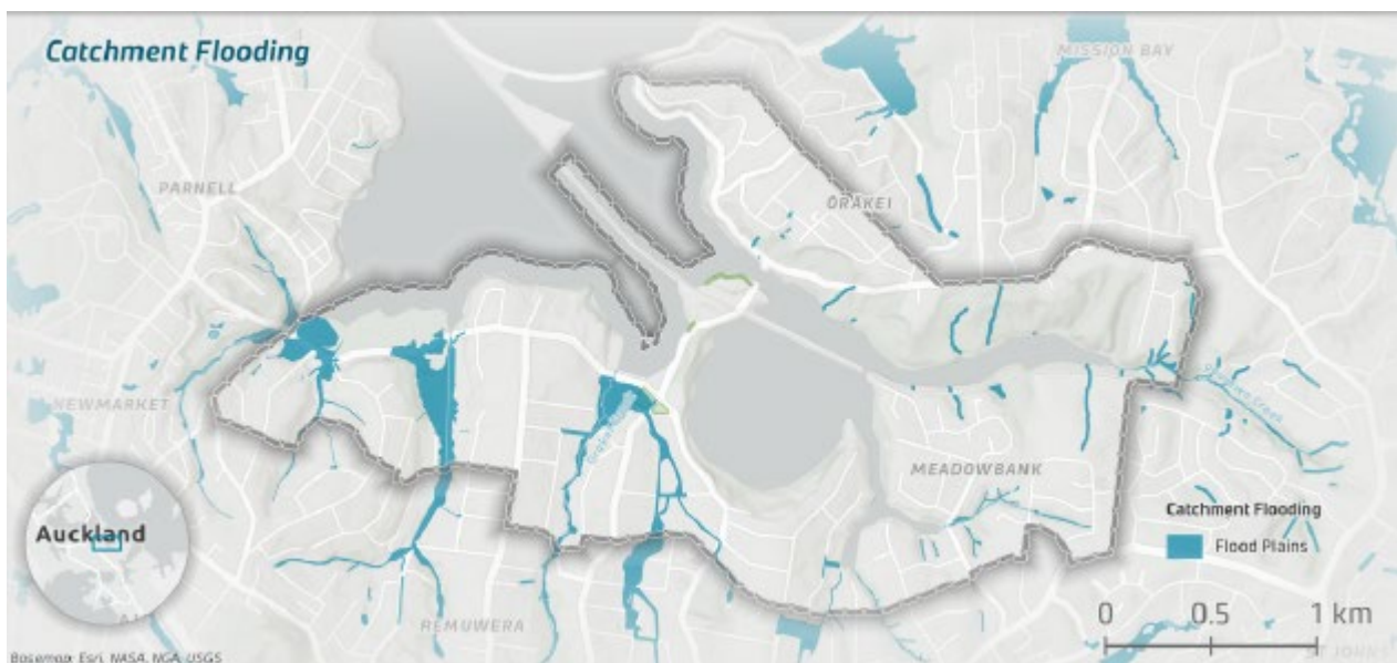
Figure 7 Catchment flooding, showing the one per cent AEP floodplains for the unit 2 area.
