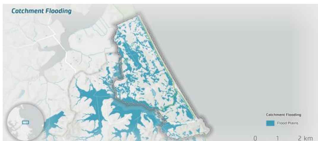
Figure 3: Coastal Hazardscape for the Te Arai Unit, reflecting coastal erosion susceptibility for 2050, 2080 and 2130 considering RCP4.5 and RCP8.5 emission scenarios, coastal inundation for 1%AEP storm surge for present day and with 0.5 m, 1 m and 2 m sea-level rise and the identification of flood plains.
