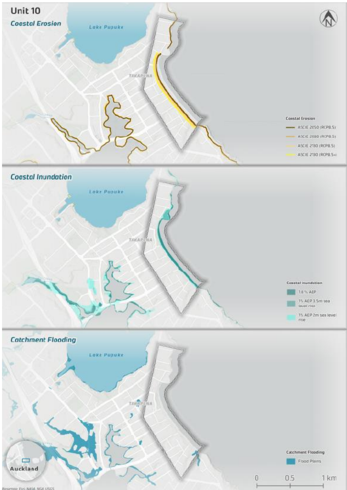
Figure 21: Coastal Hazardscape for the Takapuna Unit, reflecting coastal erosion susceptibility for 2050, 2080 and 2130 considering RCP4.5 and RCP8.5 emission scenarios, coastal inundation for 1%AEP storm surge for present day and with 0.5 m, 1 m and 2 m sea-level rise and the identification of flood plains.
