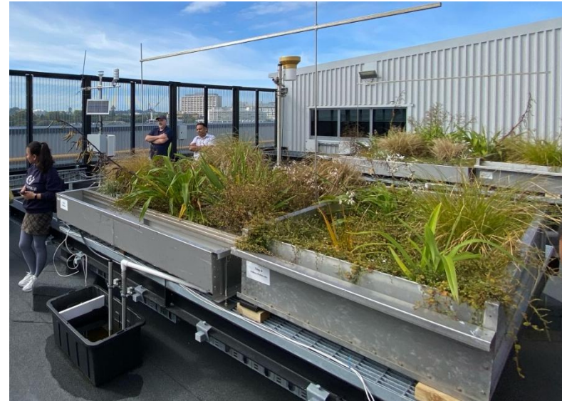
Figure 3: Living Roof test beds, University of Auckland, Engineering Roof
