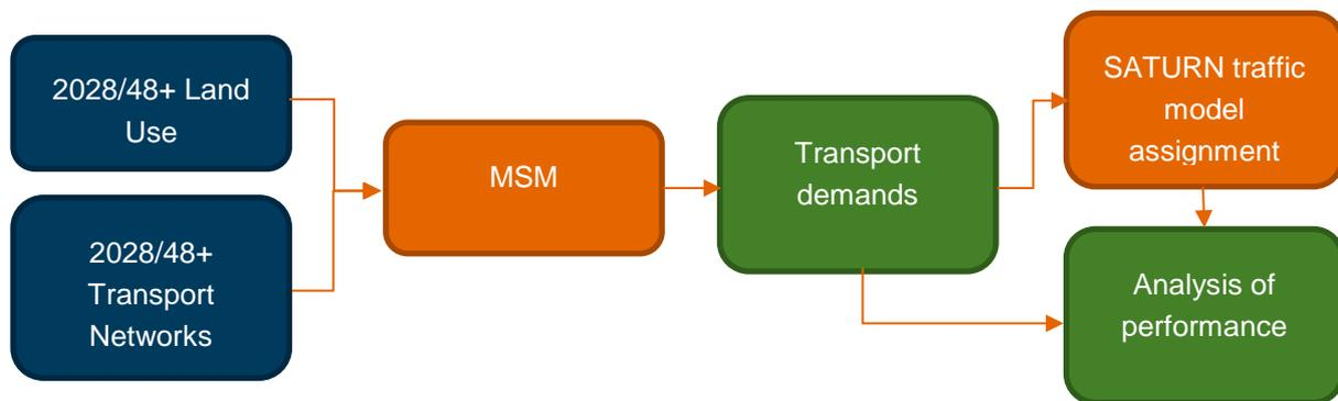
Figure 7-1 – ITA model structure.
