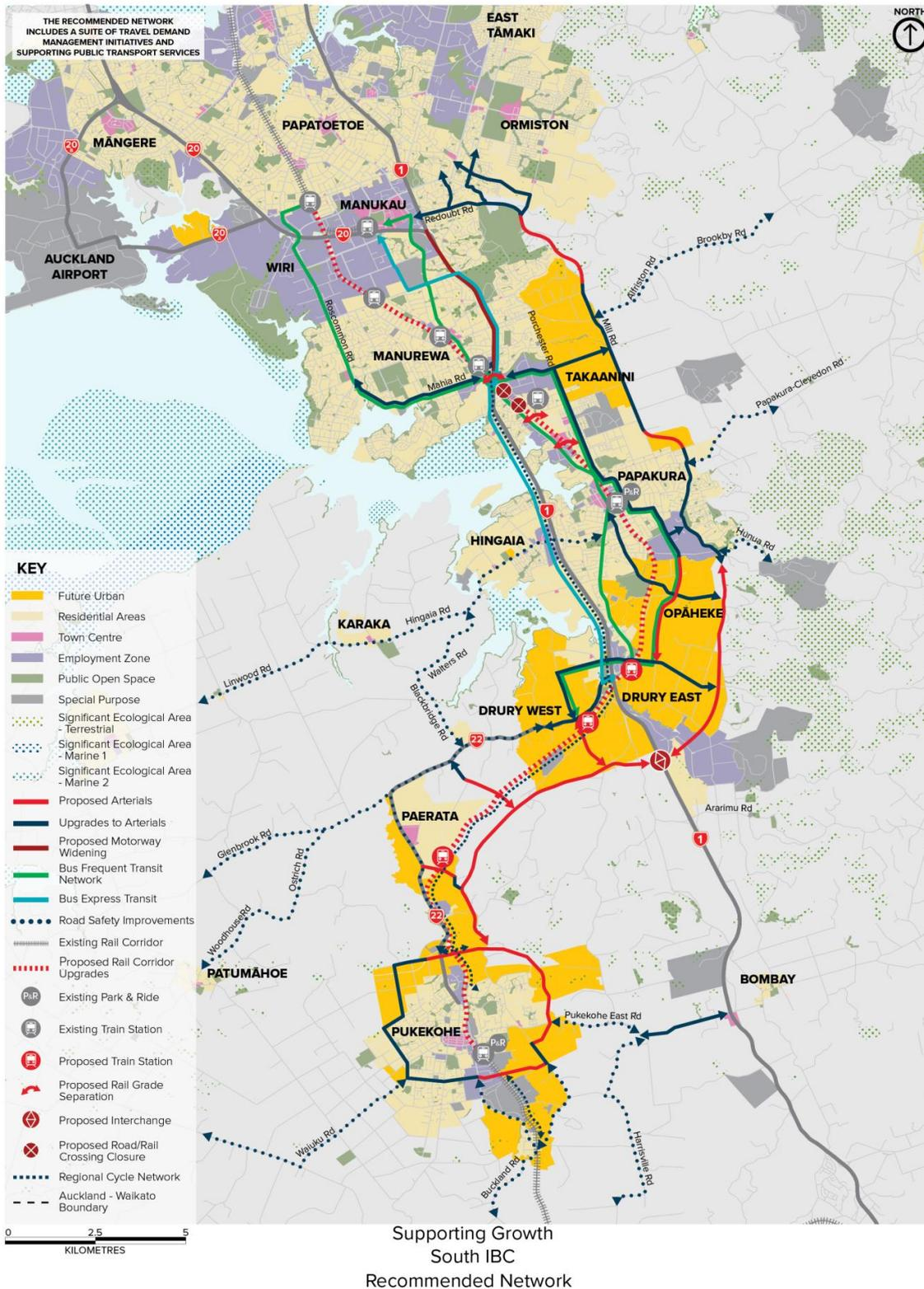
Figure 6-10 – IBC draft recommended network, with rail line labelled as the dashed red line, frequent bus & routes in green, and SH1 express bus route in blue. N.B. Pukekohe will be served mainly by feeder (connector and local) routes with rail services operating as the backbone service.
