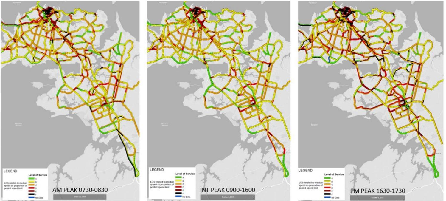
Figure 5-2 – LOS (vehicle speeds) as a proportion of posted speed limit. Study area in the bottom-right.
