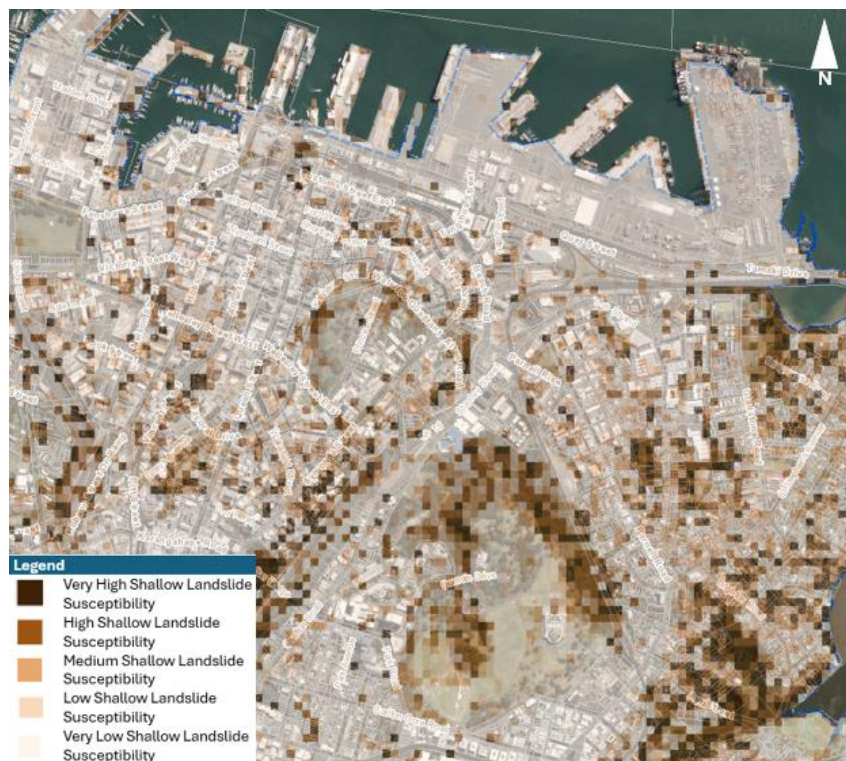
Figure 4: AUP:OP Shallow Landslide Susceptibility (Source: AUP:OP maps)
