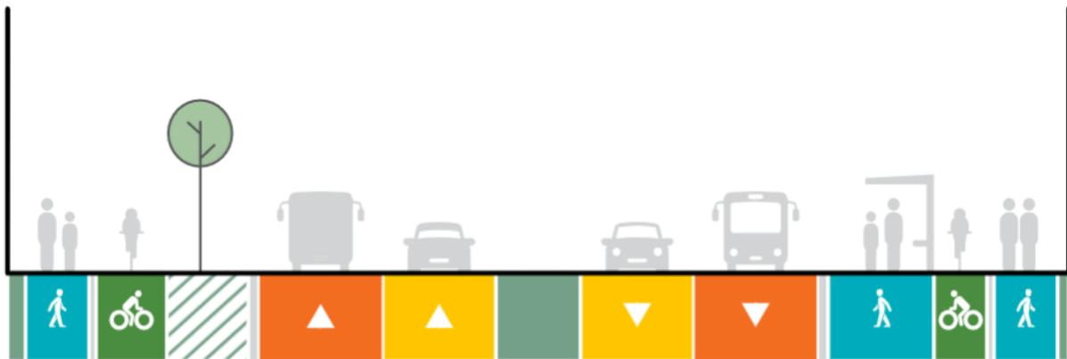
Figure 11-7: NOR RE1 Fred Taylor Drive typical 30 m cross section
