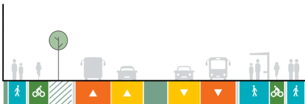
Figure 10-9: NOR W2 Māmari Road upgrade typical cross-section – corridor
