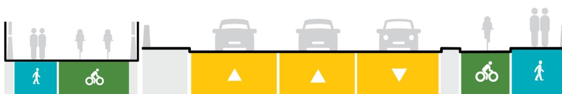
Figure 10-7: NOR W1: Trig Road (North) typical cross section – existing bridge and new active mode bridge
