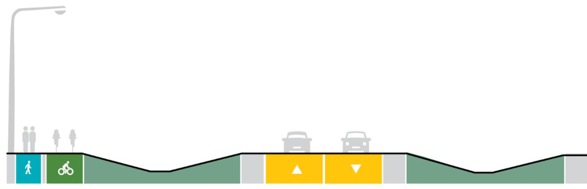
Figure 11-10: Coatesville-Riverhead Highway typical 33 m rural cross section
