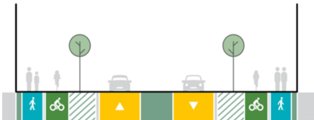
Figure 11-9: Coatesville-Riverhead Highway 24 m urban arterial
