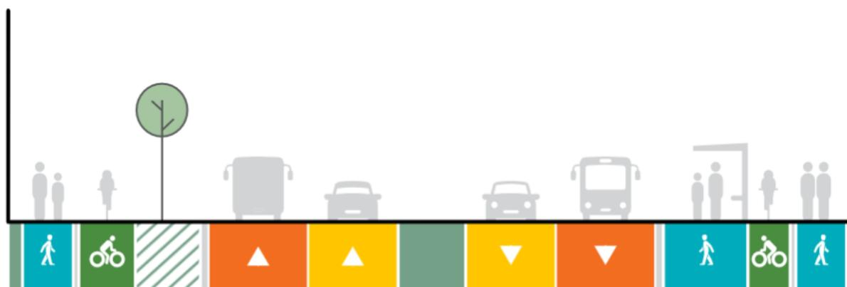
Figure 11-5: NOR RE1 Don Buck Road typical 30m cross section
