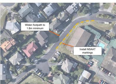
It is recommended that the new road extension within the site continues this cross section, with a 5.5m wide carriageway. The footpath width within the site should measure a minimum of 1.8m wide.
