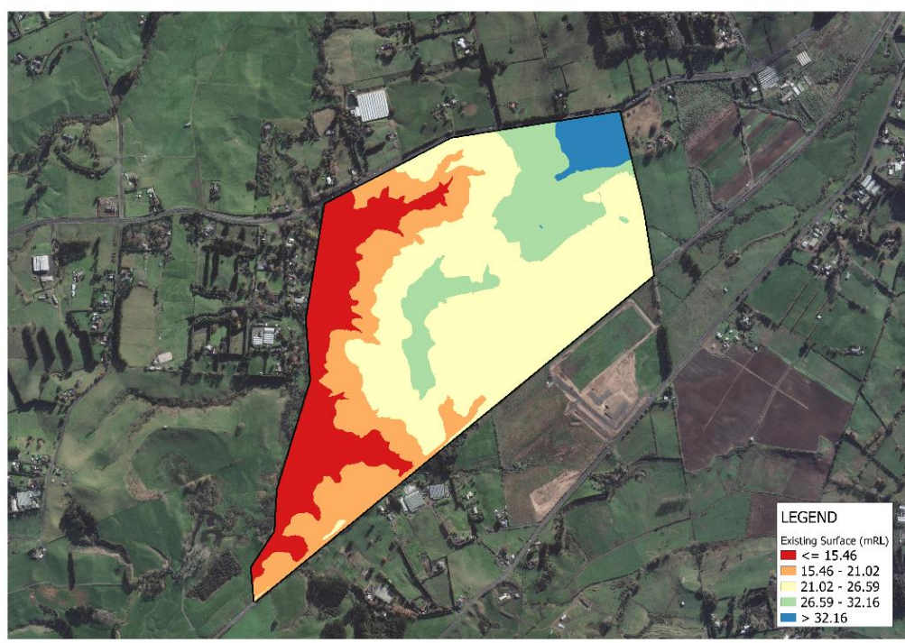
Figure 6: Site terrain (LiDAR 2016)
