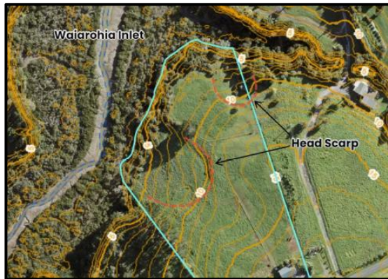
Image 1: 10 Sinton Road, two head scarps as shown
