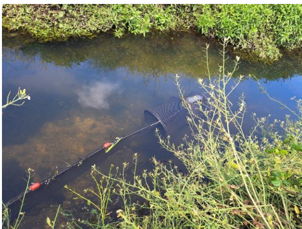
Figure 6. a) Fyke net and b) Gee's minnow trap set in the assessment reaches.
