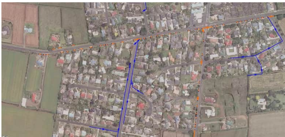
Figure 7: Conduits Type (Conduits (2D)) for small culverts only ICM 2023.2 (Orange colour)
