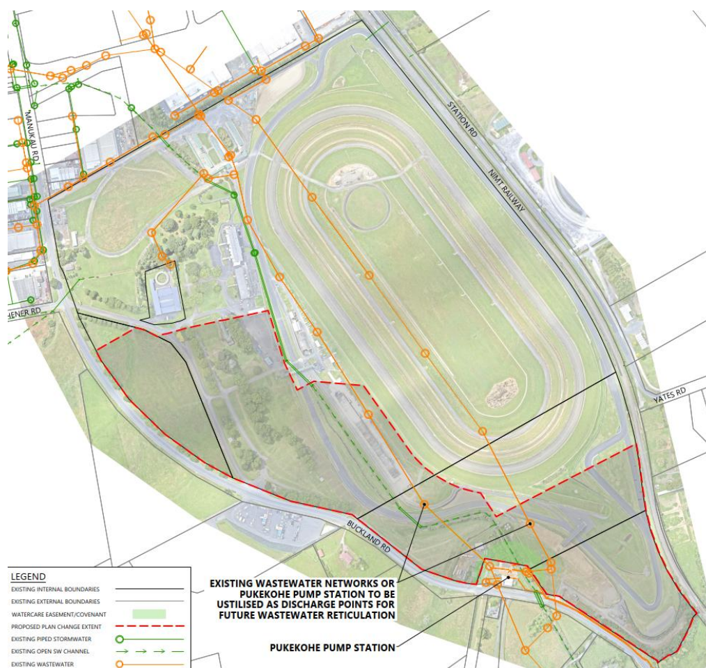
Figure 5: Wastewater Network and Potential Future Connection Points
