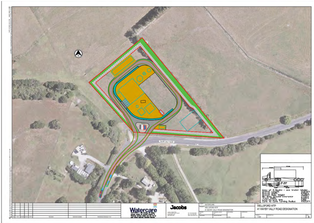
Figure 7: B-Train Heavy Commercial Vehicle Swept Path
