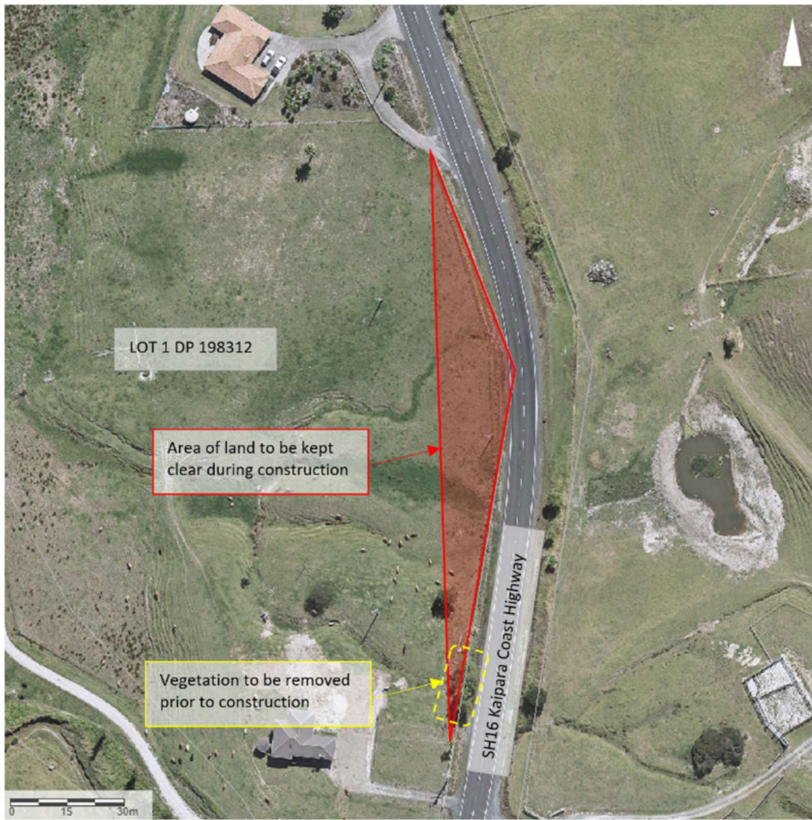
Figure 1: Vegetation to be removed prior to, and area of land to be kept clear during construction, Lot 1 DP 198312
