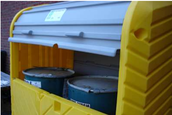
Secondary containment with cover
