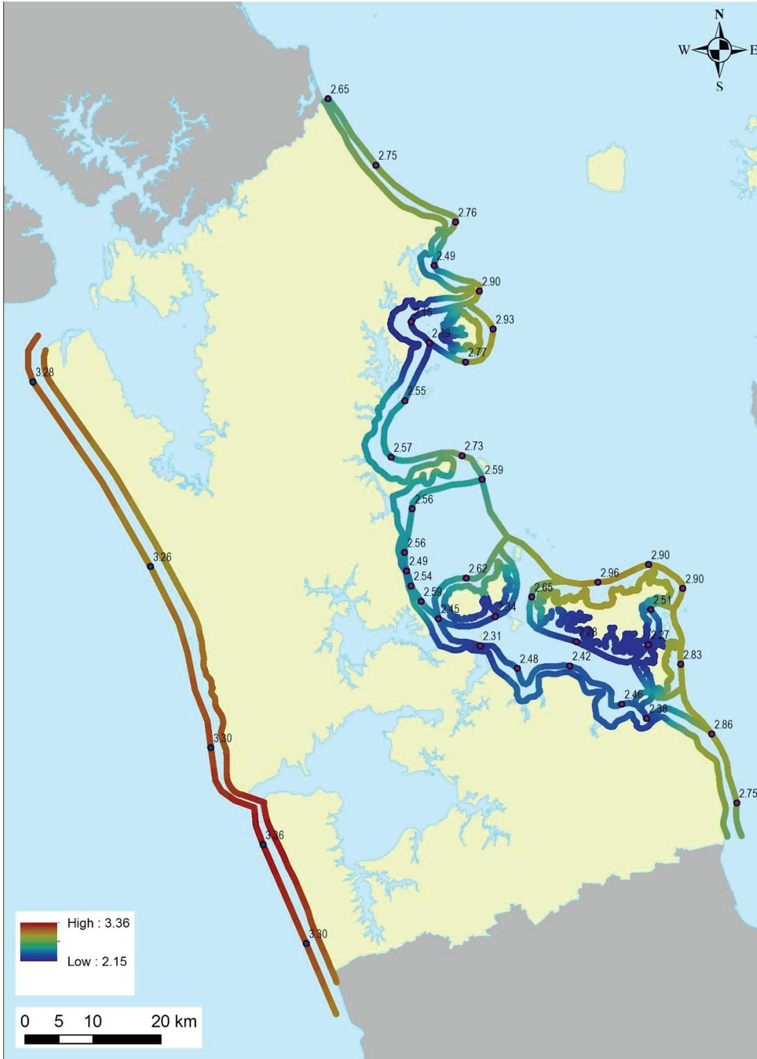
**Figure 8-2: Map of the Auckland Region with interpolated elevations on the lines connecting model output locations, and elevations transferred from offshore lines to points along the coastline.**
