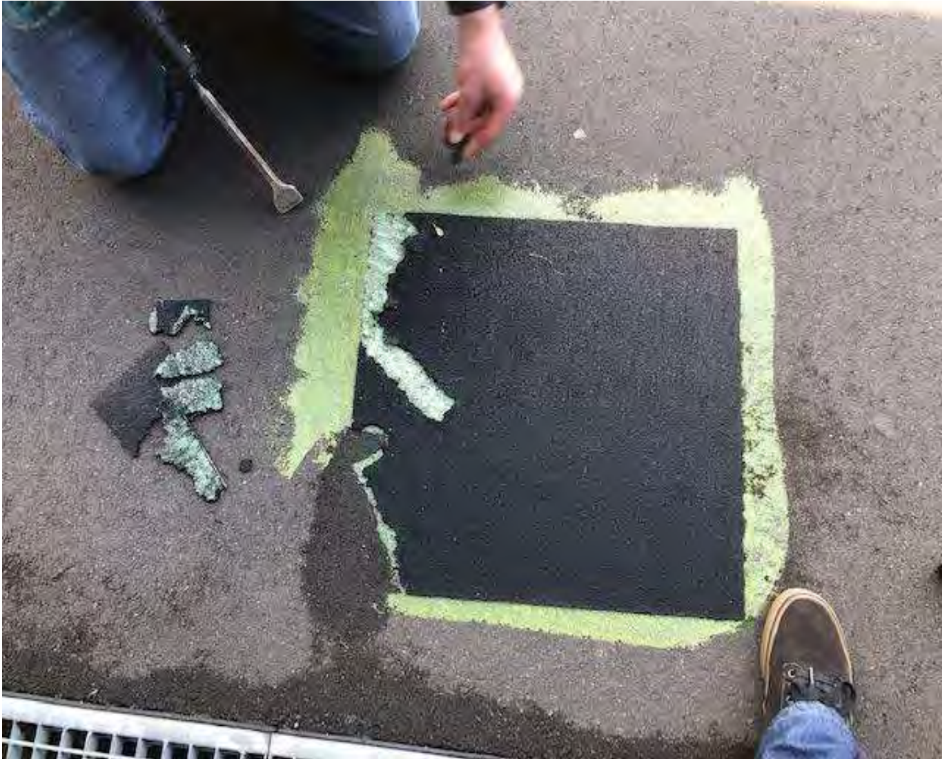
Example of an adhesion check on the surface showing the mat completely stuck to the surface and very difficult to remove.
