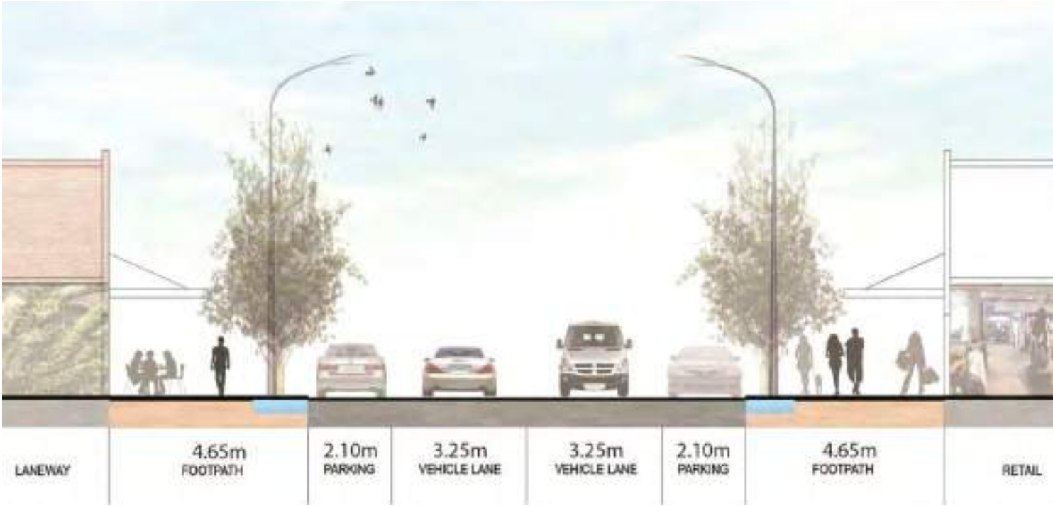
Figure 8. A possible Kitchener Road cross section (note: dimensions do not indicate a final design; the above design is subject to further design and stakeholder engagement and may comprise alternative options)
