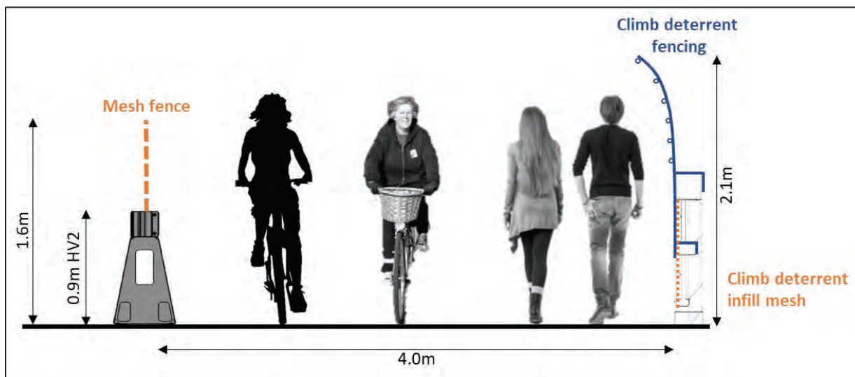
Figure 31 Proposed cross-section of Auckland Harbour Bridge Shared Path to address Waka Kotahi safety concerns (1.8m high people used for reference)
