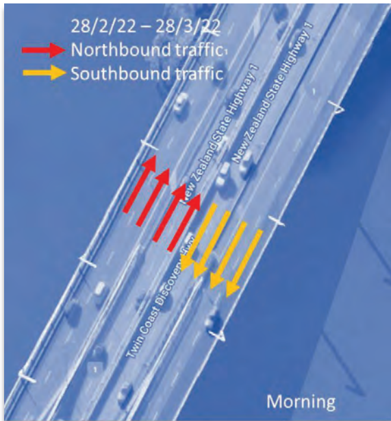
Figure 21 Feb-March 2022 4-Lane Arrangement
