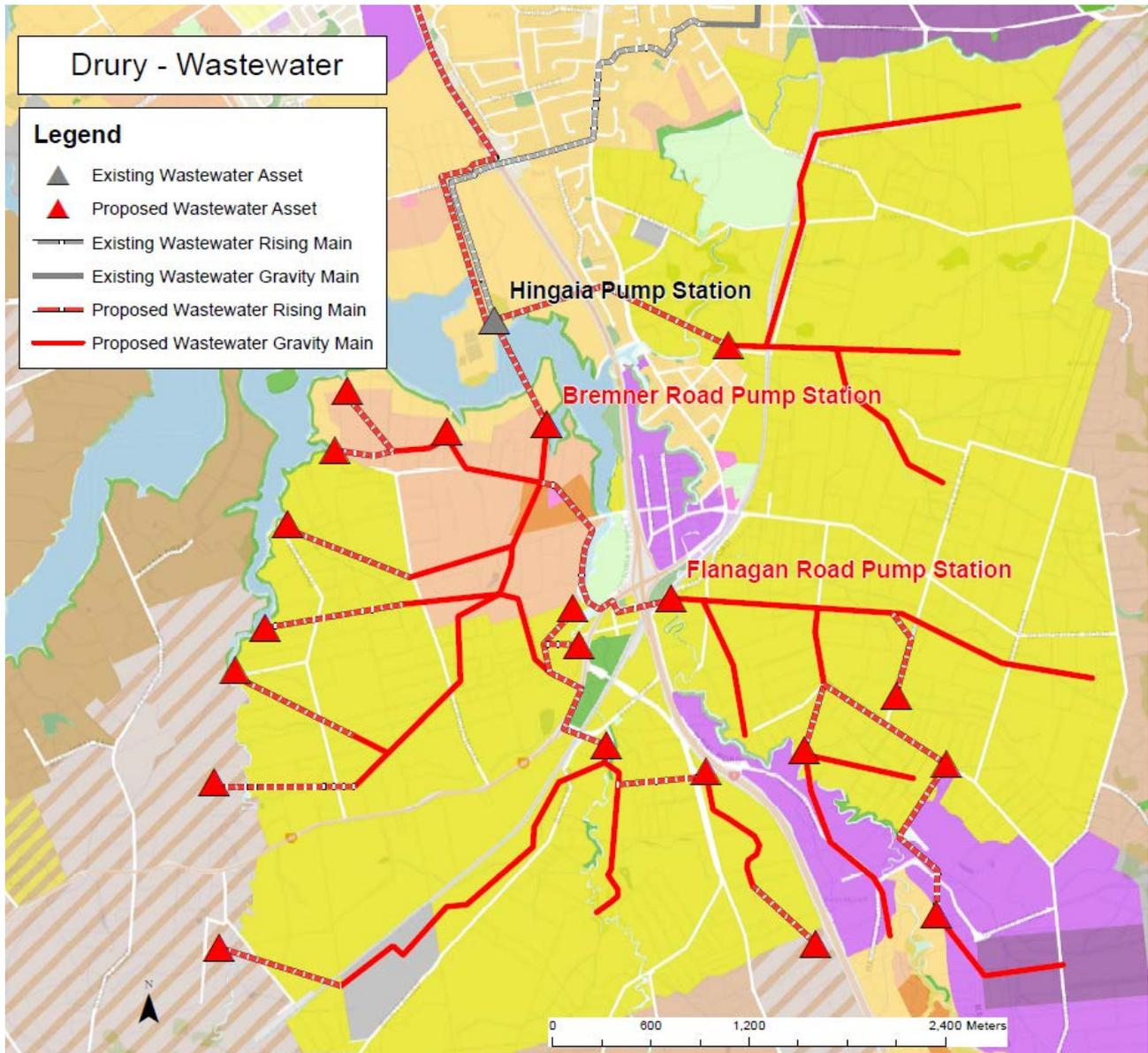
**Figure 3:** Indicative Drury – Opāheke Wastewater Servicing Plan
