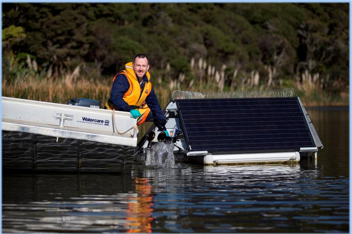
Ultrasonic technology trial to monitor and combat blue/green algae in the Lower Nihotupu Lake
