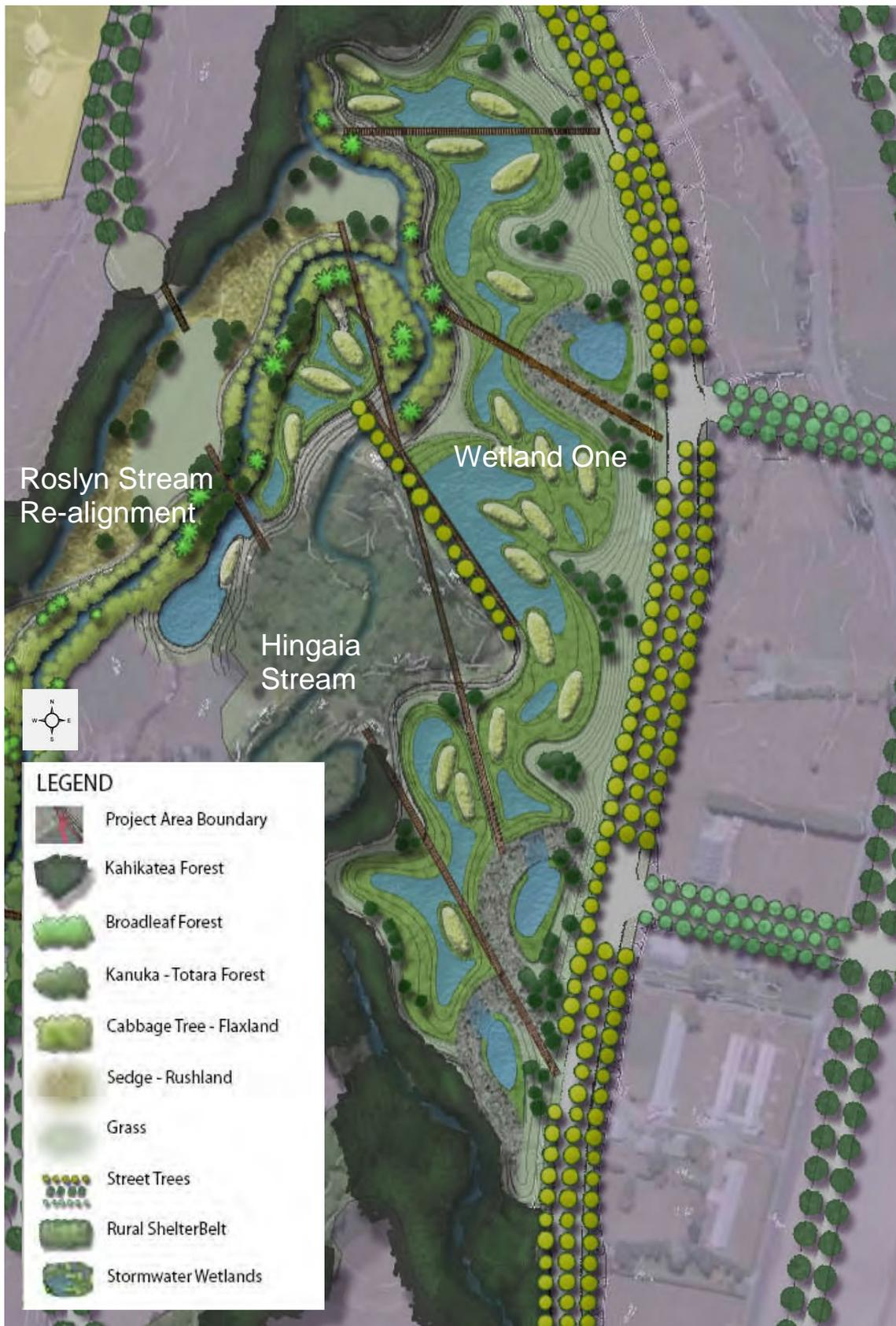
FIGURE 9: Proposed Planting Plan for Stormwater Wetland One
