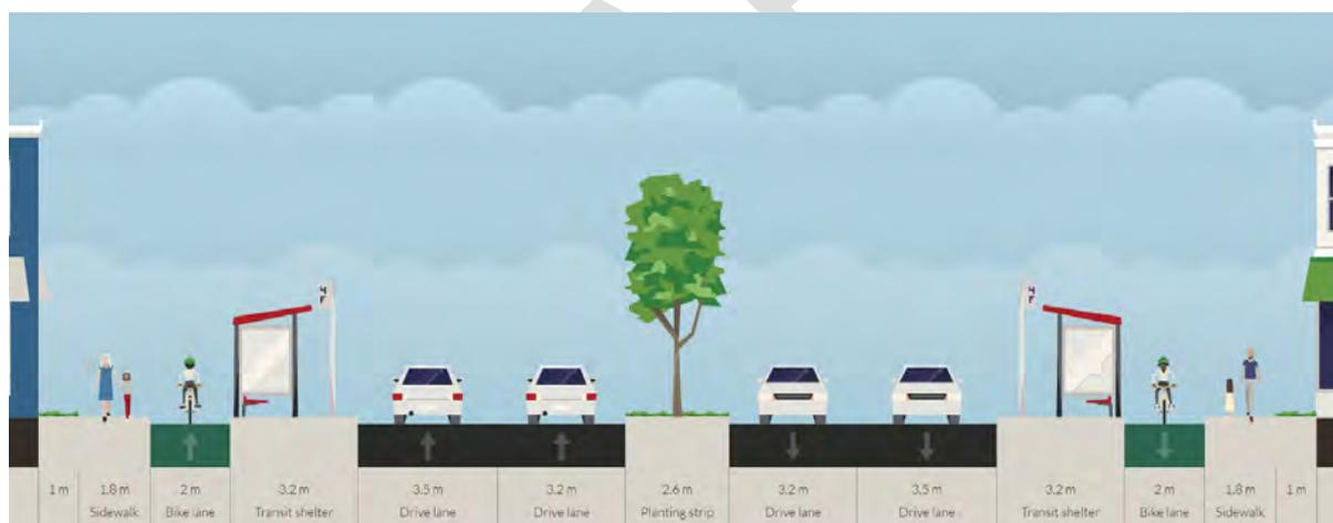
**Figure 28: Urban Arterial Bridge Indicative Cross Section**
