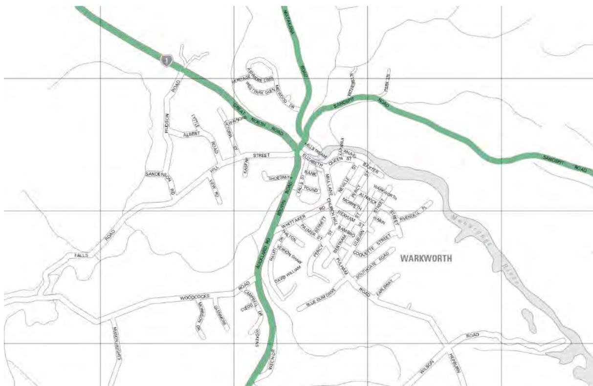
As shown above, SH1, Matakana Road and Sandspit Road are all overdimensional vehicle routes. The overdimensional routes are expected to remain post-completion of Ara Tūhono and therefore will affect any proposed intersections along these routes.
