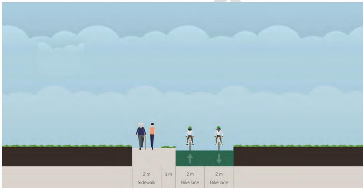
**Figure 30: Collector Road Indicative Cross Section**
