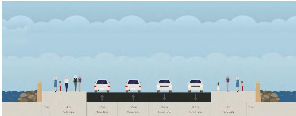
**Figure 29: Primary Walking and Cycling Corridor (Off road) Indicative Cross Section**
