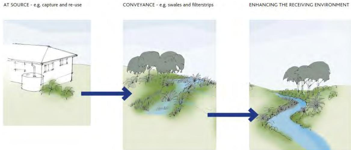
Figure 6.2: Example of a treatment train for water quantity (source: GD04 (Auckland Council, 2015))
