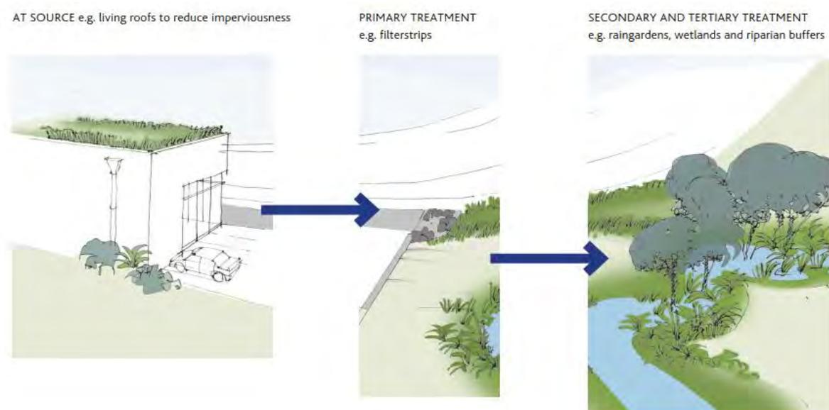
Figure 6.3: Example of a treatment train for water quality (source: GD04 (Auckland Council, 2015))
