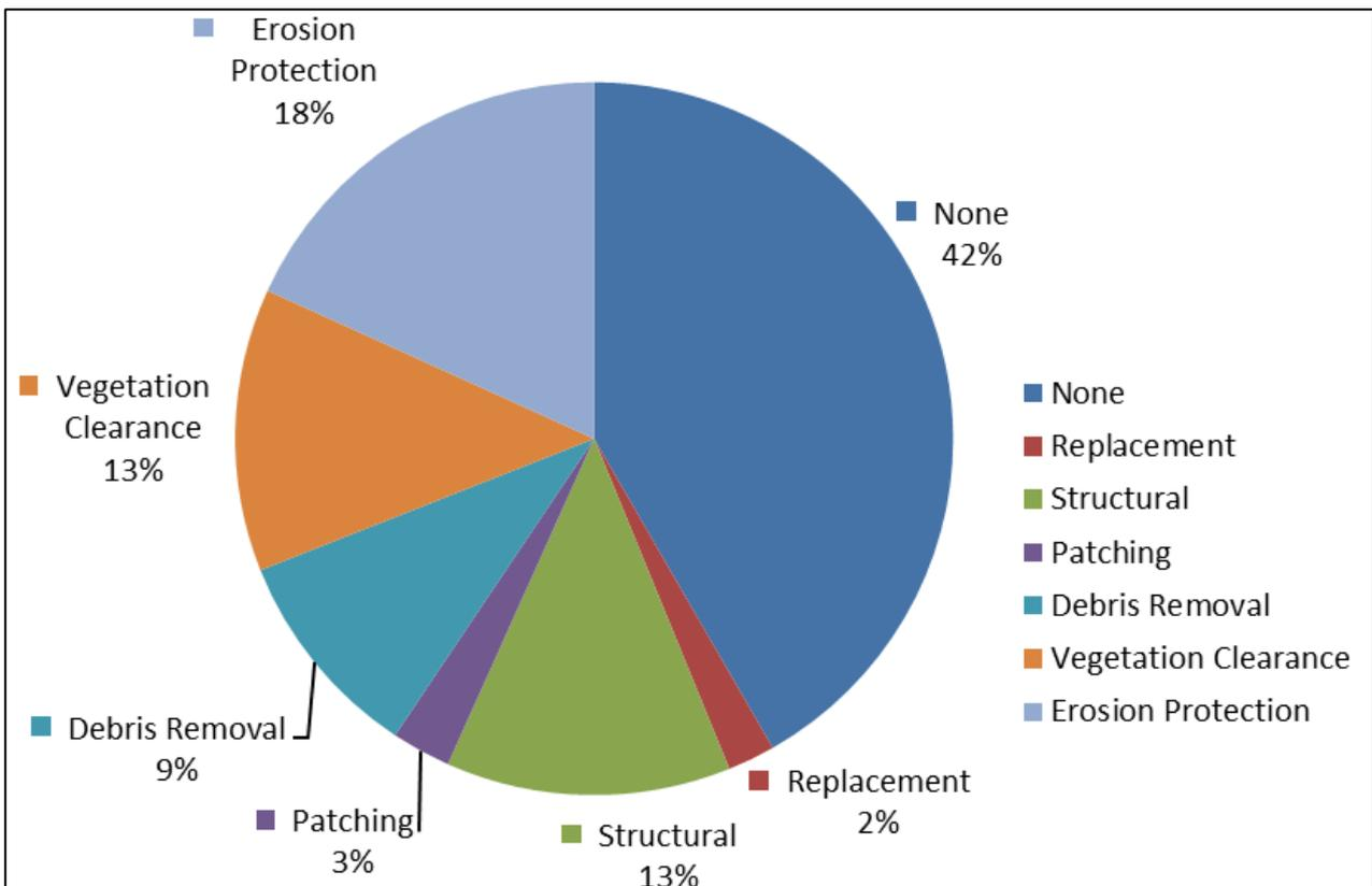
Figure 5: Oira Creek Outlets and Inlets Structures Maintenance Required Proportion (of rateable inlets/outlets).
