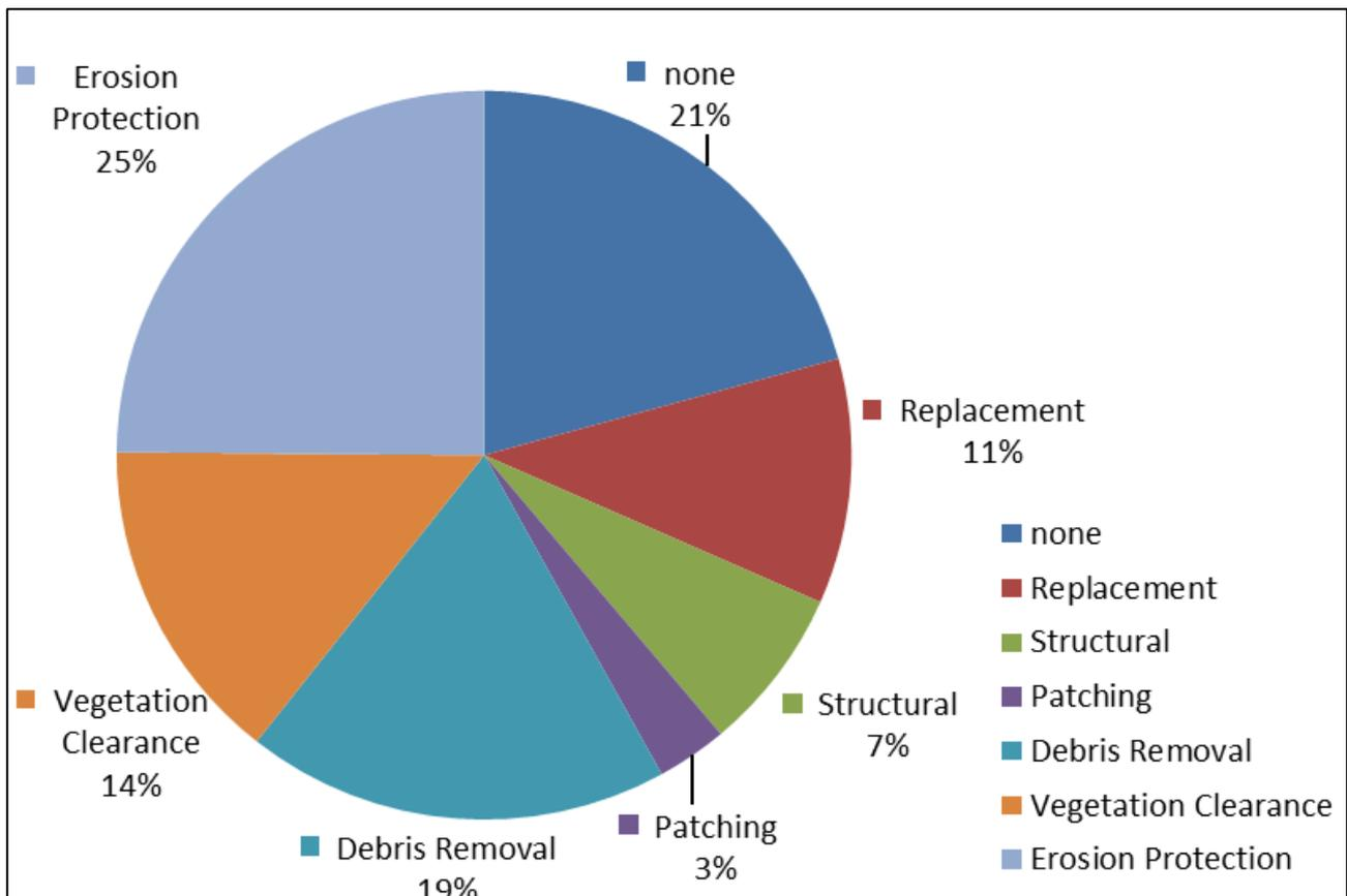
Figure 7: Oira Creek Culverts and Pipes Maintenance Required Proportion (of rateable culverts/pipes).
