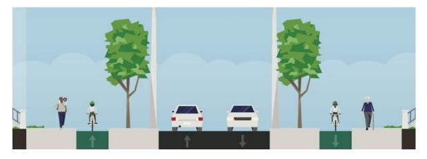
Figure 8-20 – Urban collector (21m) indicative cross-section
