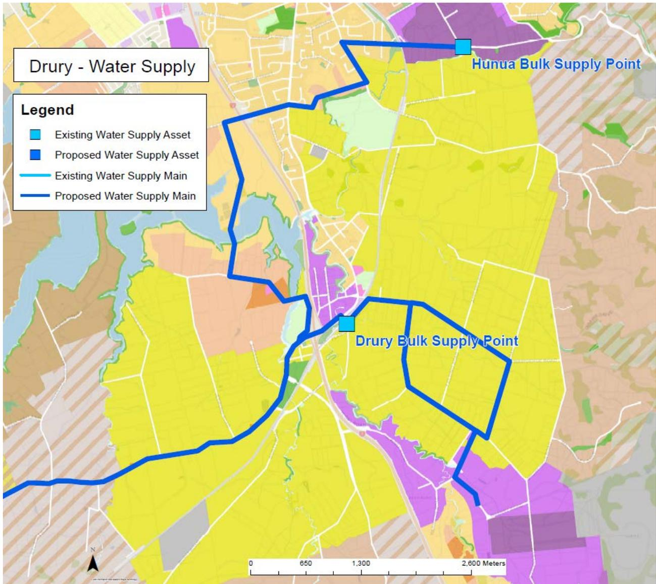
**Figure 2:** Indicative Drury – Opāheke Water Servicing Plan
