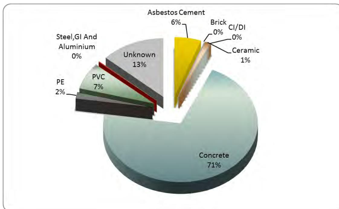
Figure 5.6 Pipes and Culvert Material
