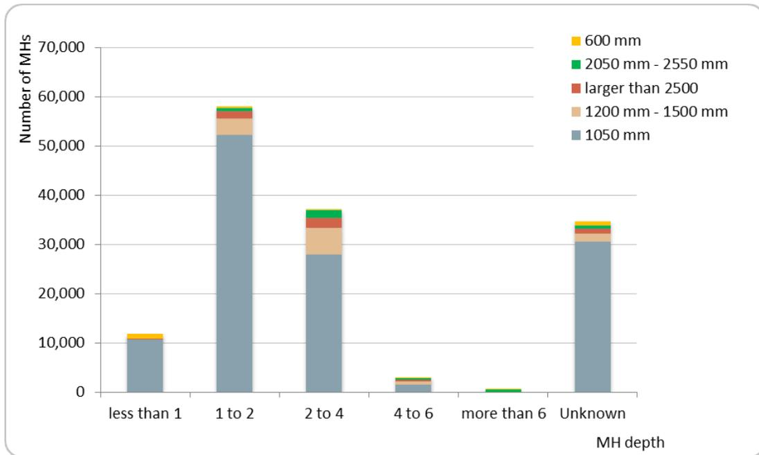
Figure 5.5 Manhole size and depth distribution
