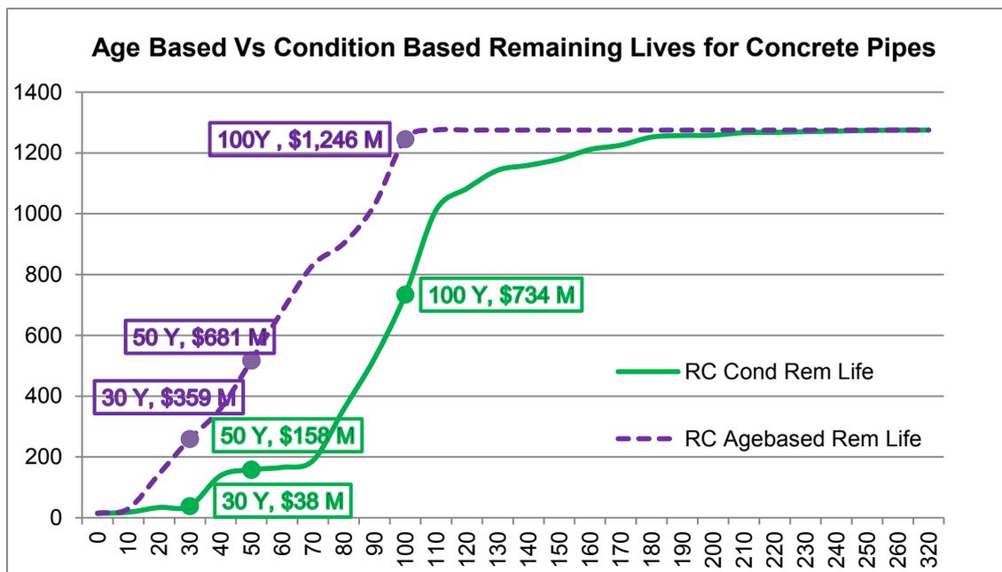
Figure 7.10 Comparison between age based and condition based remaining lives in concrete pipes
