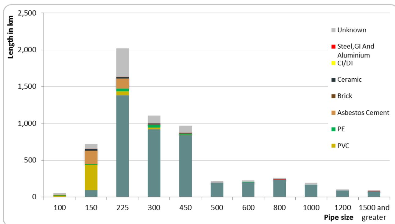
Figure 5.2 Pipe diameters, lengths and material
