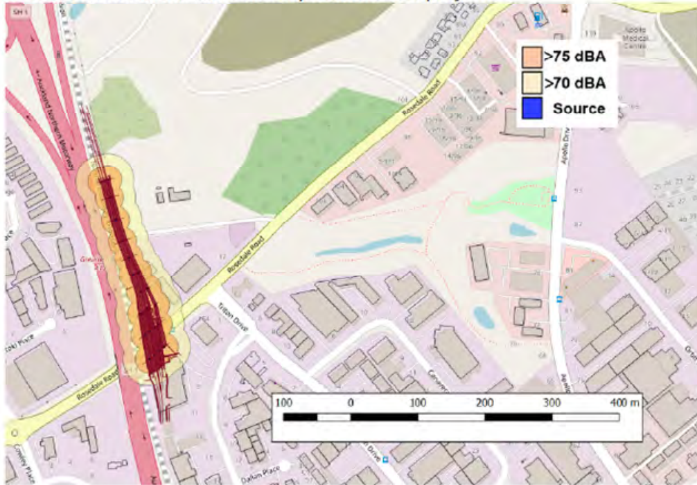
Figure 1: Noise contours from vibratory pile driving, calculated from actual noise measurements of the same activity from the NCI project.
