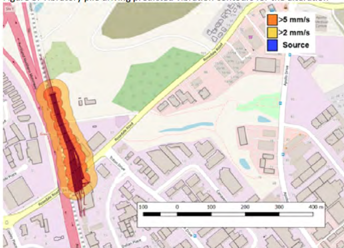
Figure 3: Vibratory pile driving predicted vibration contours for the alteration
