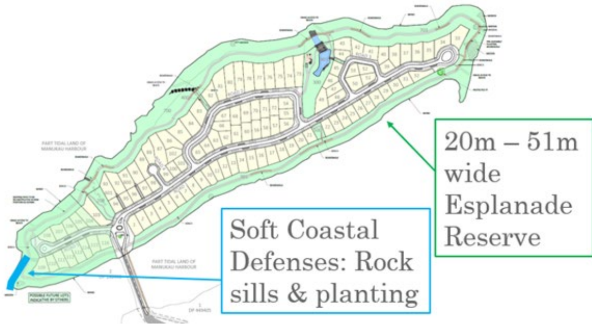
Figure 48: Plan showing agreed extended esplanade reserve to address coastal erosion over the long-term: Pararaekau island, Manukau Harbour (Source: Auckland Council)
