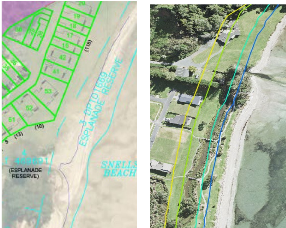
Figure 49: Esplanade reserve land at Snells Beach as measured from MHWS in 2017 [left] and areas identified as susceptible to coastal erosion over different time periods [right] (Source: Auckland Council)
