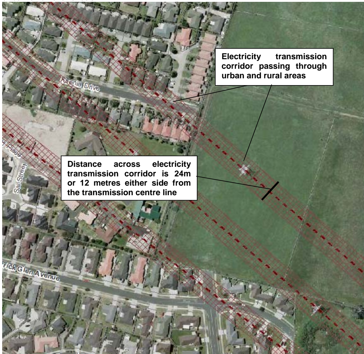
Figure 1: Aerial map depicting the electricity transmission corridor passing through urban and rural areas
